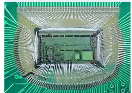
Figure 2. Real-life example of pad sizing, wire lengths and layout.
