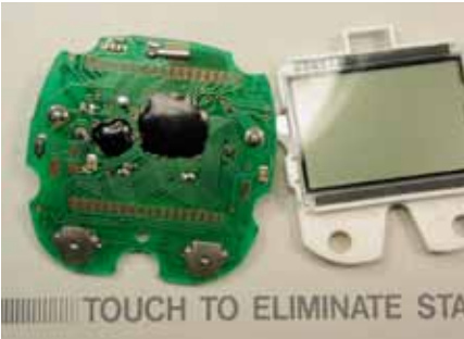
Figure 10. COB devices in a microwave oven modules.
